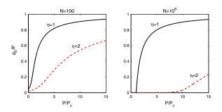
FIG. 1 (color online). The fraction of power in the first eigenmode  $p_0/P$  versus the normalized total power  $P/P_c$  for  $\eta = 1$ (solid black line) and  $\eta = 2$  (dashed red line). The left figure is calculated for N = 100, and the right for  $N = 10^6$ , shows for  $\eta = 1$  a sharp BEC transition at  $P = P_c$ , and for  $\eta = 2$  a gradual population buildup.
