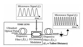
Fig. 1. Schematic of the proposed microwave frequencyshifting technique based on a general temporal selfimaging (Talbot) effect.
