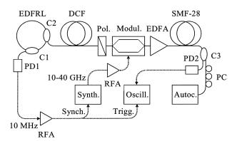
Fig. 2. Experimental setup: EDFA, erbium-doped fiber amplifier; C3, fiber coupler; PC, polarization controller; other notation defined in text.
