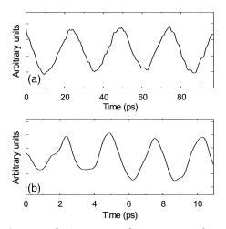
Fig. 4. Autocorrelation traces that correspond to the optical signals measured (a) before and (b) after the second dispersive stage when the TI system is configured for achieving  $M_t = 0.113$ , with  $f_1 = 40$  GHz.
