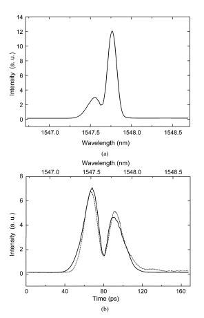
Fig. 3. Experimental results. (a) Measured spectrum of the input pulse to the time lens. (b) Measured spectrum of the output pulse from the time lens (solid curve, top scale) and measured temporal waveform of the input pulse to (output pulse from) the time lens (dotted curve, bottom scale).
