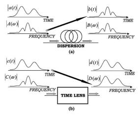
Fig. 1. Dual Fraunhofer regimes: (a) frequency-to-time conversion using dispersion and (b) time-to-frequency conversion using a single time lens.
