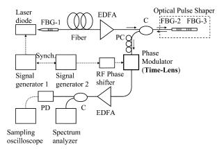
Fig. 2. Schematic of the experimental setup. Solid (dotted) lines are used for optical (electrical) signals. EDFA: Erbium-doped fiber amplifier. C: fiber coupler. PC: polarization controller. Synch.: synchronization.
