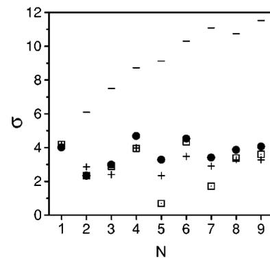
FIG. 5. Experimental spatial frequency intensity width  $\sigma$  after each of the nine gratings (closed circles) compared with the theoretical results of Eq. (1) near antiresonance (+), with  $\gamma = 2.97\pi$ , and away from antiresonance (-), where  $\gamma = \sqrt{5} - 1$ . The results of the linear model (2), marked by squares, are presented as well.
