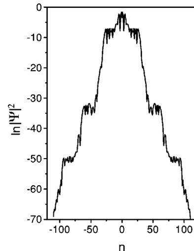
FIG. 3. Typical numerically calculated confined spatial frequency spectrum  $|\psi|^2$  near antiresonance, with  $\gamma = 2.97\pi$  (or  $\delta = -0.03$ ), after  $N = 200$  kicks, having a “fir-tree” shape.
