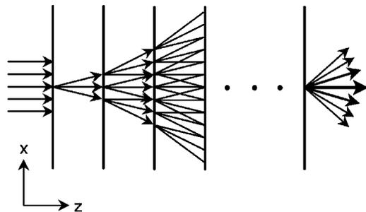
FIG. 1. Schematic description of the free space “kicked” optical system with the array of phase gratings having an identical spacing between them. Some of the light paths are shown.
