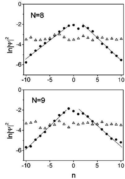
FIG. 4. Experimental confined spatial frequency spectrum intensity after the eighth and ninth gratings for the ordered (closed circles) and disordered (open triangles) gratings. The initial state (direction) is  $n=0$ , within experimental accuracy.
