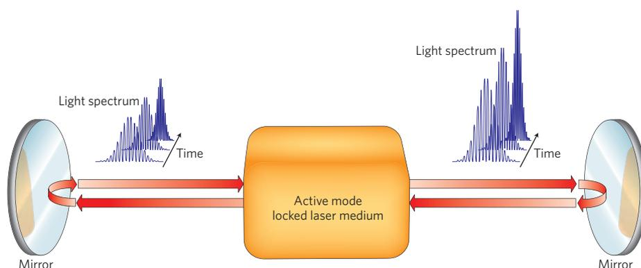
**Figure 1** | The proposed set-up for observing light condensation. A suitable active mode-locked laser amplifies and modulates an incoherent spectrum composed of many laser modes in time. As soon as the overall light power in the cavity exceeds a certain threshold, a condensation process is expected to occur: at every round trip each mode transfers a fraction of its power to a single mode, thus shrinking the overall spectrum, condensing light energy and resulting in single-mode lasing.
